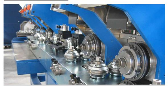
The fabrication of a Flux Cored Electrode begins by slitting steel coiled sheet into strips. The strips are passed through rollers that form it into a U-shaped cross-section. In the same operation, the formed strip is filled with a measured amount of core ingredients. The U-shaped strip is passed through closing rolls, forming it into a tube and tightly compressing the granular core material.
